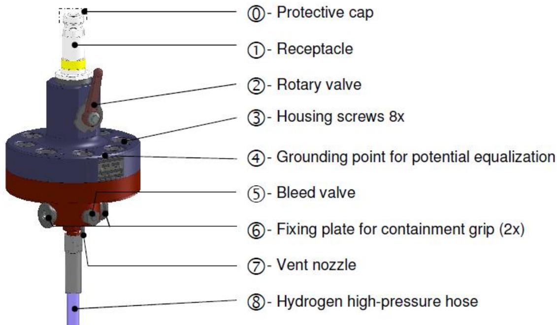
Figure 3. HYDAC PSA-H70 particulate sampler.
