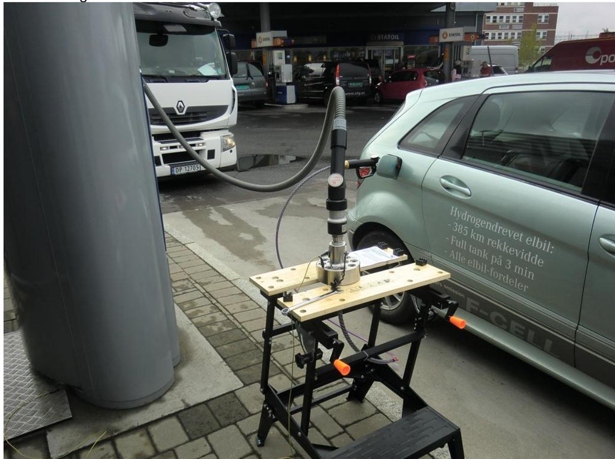
Figure 4. PSA-H70 sampler installed at HRS Økern in Oslo, Norway.
