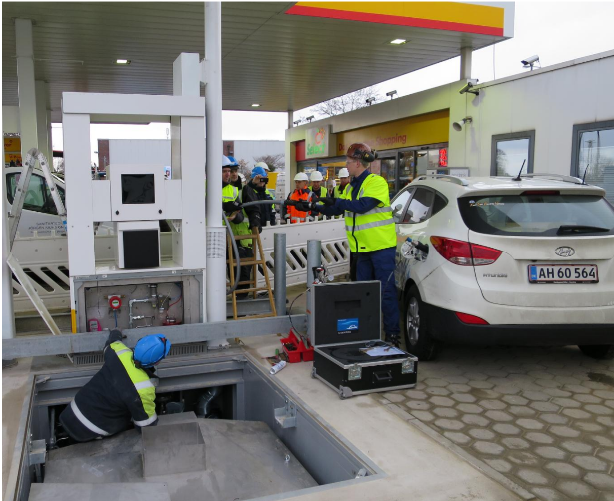
Figure 2. Sampling at H2 Logic HRS in Hamburg. The HRS was under commissioning.
